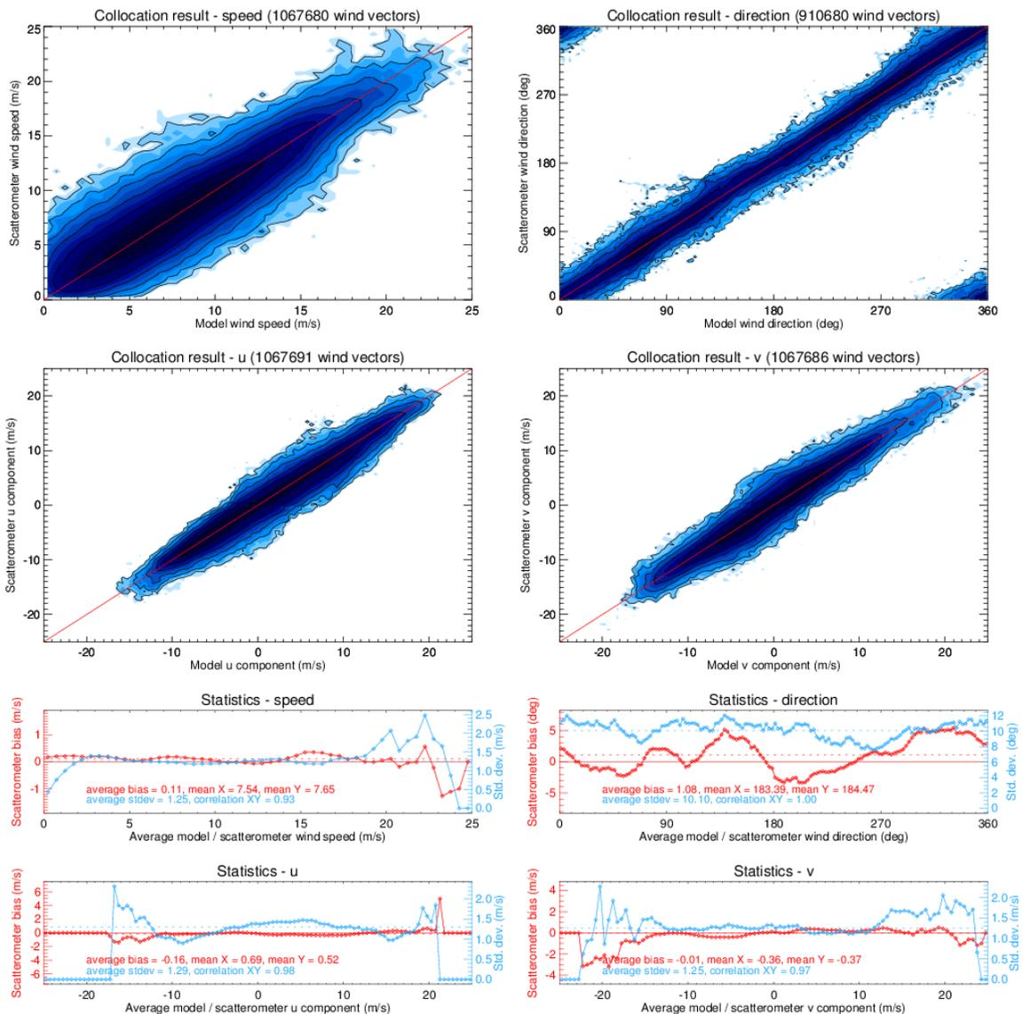
**Figure 2: Two-dimensional histograms of wind speed, direction (w.r.t. wind coming from the North),  $u$  and  $v$  components of 25 km RapidScat wind product versus the ECMWF model forecast winds from 25 and 26 January 2015 (top panels). The corresponding biases (red) and standard deviations (blue) as a function of the average scatterometer and model winds are shown in the bottom.**
