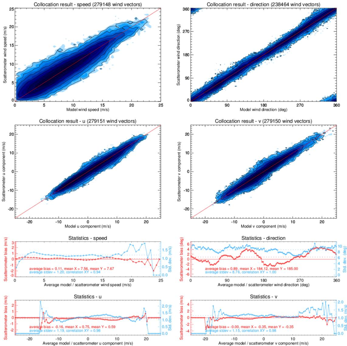
**Figure 3: Two-dimensional histograms of wind speed, direction (w.r.t. wind coming from the North),  $u$  and  $v$  components of 50 km RapidScat wind product versus the ECMWF model forecast winds from 25 and 26 January 2015 (top panels). The corresponding biases (red) and standard deviations (blue) as a function of the average scatterometer and model winds are shown in the bottom.**
