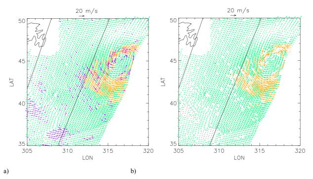
Figure 33 QuikSCAT wind fields. The colors represent the different categories: green is category A, yellow is B, purple is C, and red is D. Plot a shows all retrieved winds while plot b shows only KNMI QC accepted winds. The black solid lines separate different regions of the swath. In this case, the left side of the plot corresponds to the sweet-right region, the middle to the nadir region and the right side to the sweet-left region. The acquisition date is February 14 2001 at 22 hours UTC
