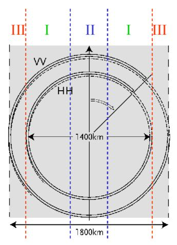
Figure 1 Schematic illustration of the QuikSCAT swath. The circles represent the two scanning rotating antennae with H-pol (HH) and V-pol (VV), and 54° and 46° incidence angles respectively. Areas I, II and III represent parts of the swath with different wind retrieval skill. Adopted from Stoffelen (1998).
