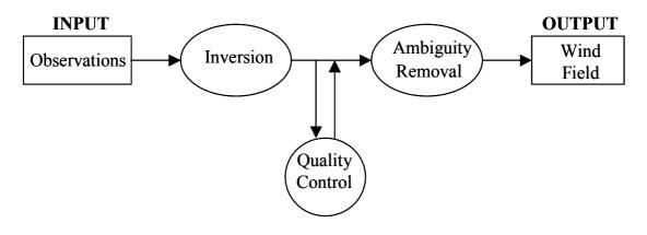
Figure 2 Schematic illustration of the scatterometer wind retrieval process
