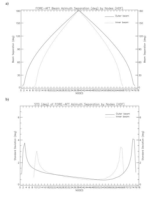
Figure 3 a) Mean fore-aft azimuth separation by node for one revolution of HDF data; the outer beam separation is in solid line and the inner beam separation in dotted line; b) Standard Deviation of the azimuth separation.
