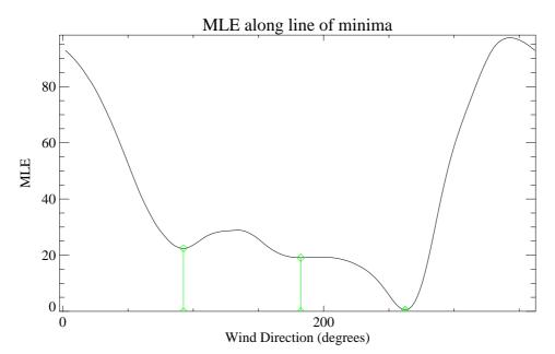
Figure 35 Example of MLE cost function for QuikSCAT WVC number 33. The green diamond symbols indicate the locations of the minima found by the inversion procedure.
